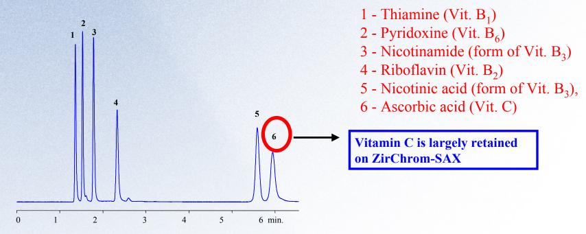
LC Conditions: Column: ZirChrom®-SAX, 150 x 4.6 mm i.d. (part number: ZR06-1546), Mobile Phase: 50 mM Ammonium dihydrogenphosphate, pH 4.5, Flow rate: 1.0 ml/min. Temperature: 30 °C, Injection Vol.: 5.0 µl, Detection: UV at 254 nm
