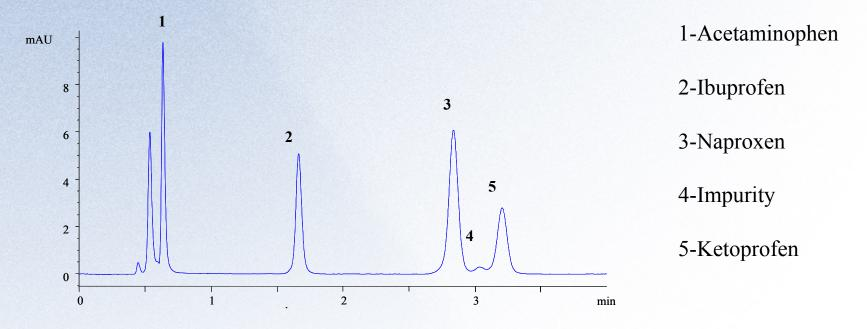
LC Conditions: Column: ZirChrom®-SAX, 50 x 4.6 mm i.d. (part number: ZR06-0546), Mobile Phase: 80/20 ACN/15 mM ammonium formate, pH=4.0 (adjusted with formic acid), Flow rate: 1.0 ml/min. Temperature: 35 °C, Injection Vol.: 1.0 µl, Detection: UV at 254 nm
