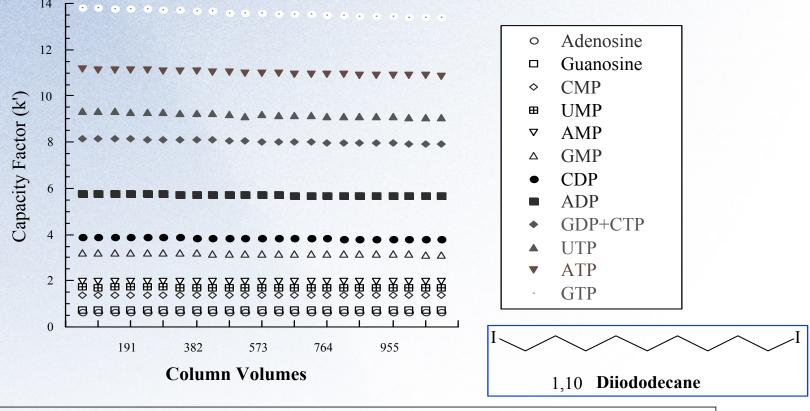
mobile phase, A =0.01M potassium phosphate dibasic, 0.04M NaCl @ pH 7.0, B = ; 0.1M potassium phosphate dibasic, 0.4M NaCl @ pH 7.0; gradient, 10% B to 90% B over 25min; injection volume, 5  $\mu$ l; column temperature, 75°C; UV detection @ 240 nm
