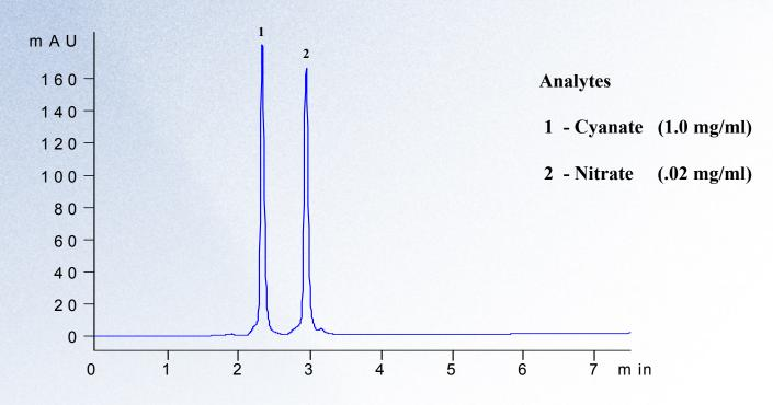
LC Conditions: Column: ZirChrom®-SAX, 150 x 4.6 mm, Flow rate: 1.0 mL/min. Temperature: 30°C, Detection: 205 nm, Injection volume: 5 ul, Mobile Phase: 25mM sodium fluoride, 175mM sodium chloride at pH 10.0
