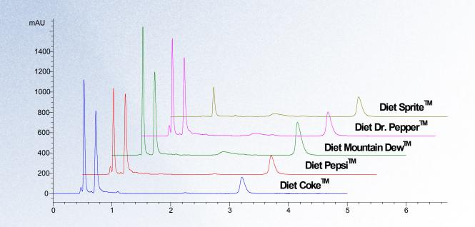
LC Conditions: Column: 3.0 mm x 100 mm ZirChrom®-SAX, Mobile Phase: 10mM Ammonium phosphate, 5mM Ammonium carbonate, pH 6.6, Flow rate: 1.0 ml/min, Temperature: 50 °C, Injection Vol.: 5.0 µl, Pressure Drop: 205 bar Detection: UV at 210 nm.
