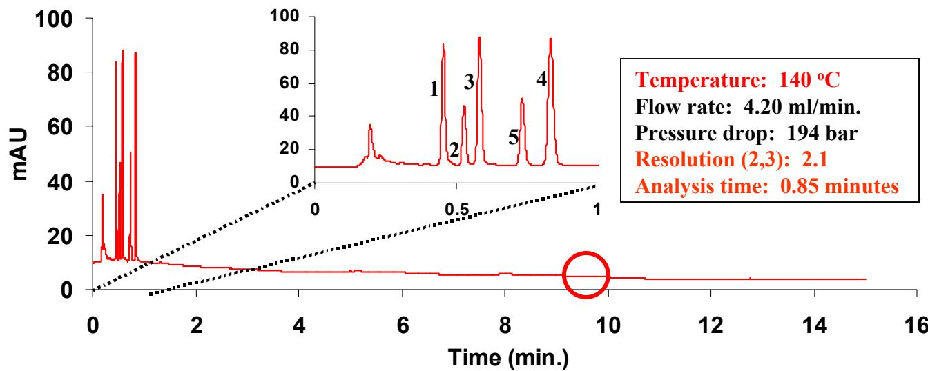
Mobile Phase, 29/71 ACN/50mM Tetramethylammonium hydroxide, pH 12.2; Injection volume, 0.5  $\mu$ l; 254 nm detection; Solutes: 1=Doxylamine, 2=Methapyrilene, 3=Chlorpheniramine, 4=Triprolidine, 5=Meclizine; Column, 100 mm x 4.6 mm i.d. ZirChrom®-PBD
