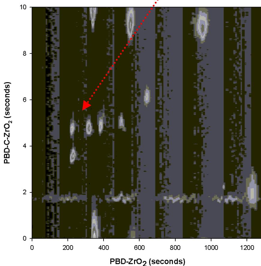
**1<sup>st</sup> Dimension Conditions:** Column, 50 mm x 2.1 mm i.d. PBD-ZrO<sub>2</sub>; Mobile phase, 20/80 ACN/Water; Flow rate, 0.08 ml/min.; Injection volume, 20 µl; Temperature, 40 °C
