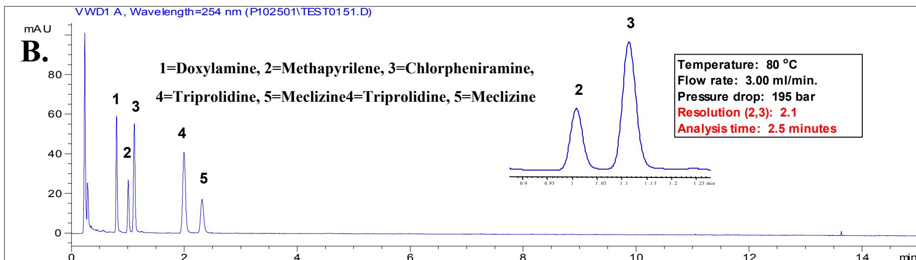
LC Conditions: (A) Mobile Phase, 29/71 ACN/50mM Tetramethylammonium hydroxide; Injection volume, 0.5  $\mu$ l;
