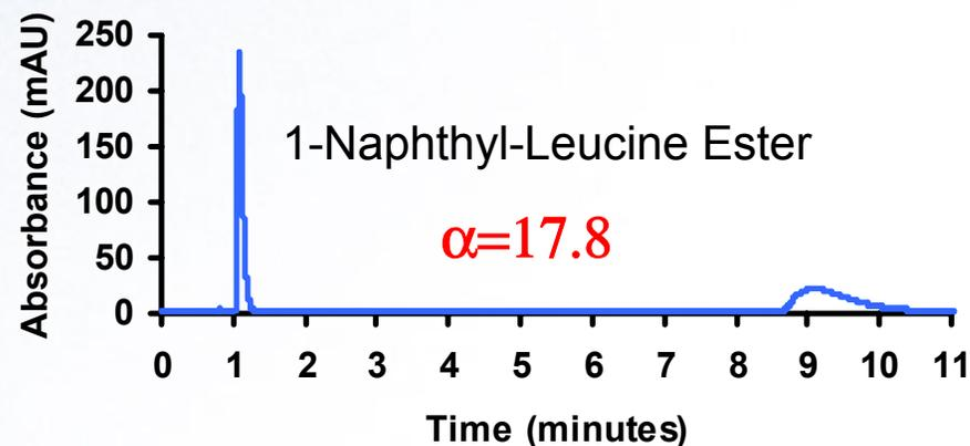
Selected Chromatograms of Chiral Compounds on Zirconia Based DNB-L-LEU Anchored with APPA.
