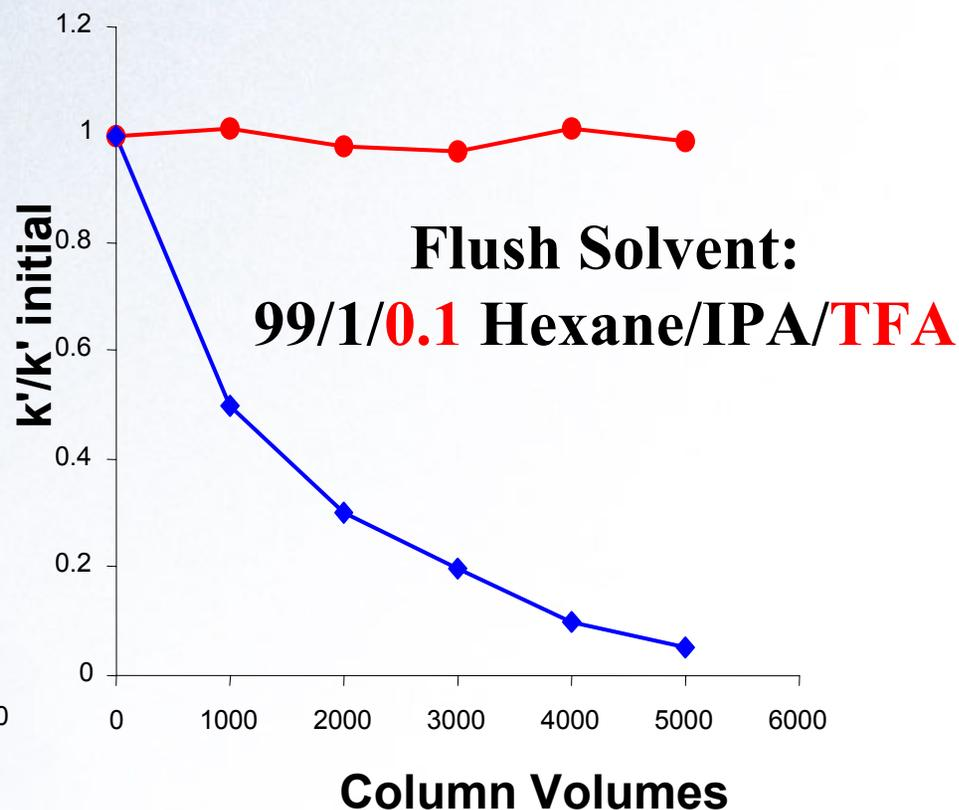
Test solute: trifluoranthryl ethanol. Note that the retention factor ratio is for the less retained isomer.
