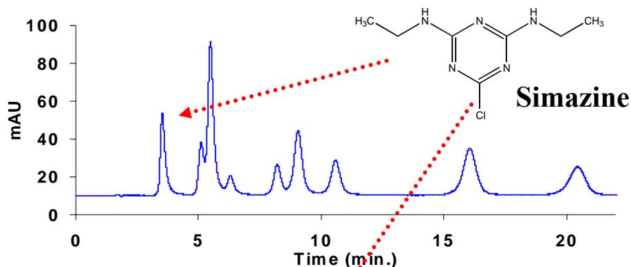
**1<sup>st</sup> Dimension Conditions:** Column, 50 mm x 2.1 mm i.d. PBD-ZrO<sub>2</sub>; Mobile phase, **20/80 ACN/Water**; Flow rate, 0.08 ml/min.; Injection volume, 20 μl; Temperature, 40 °C
