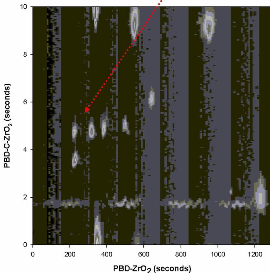
**2<sup>nd</sup> Dimension Conditions:** Column, 50 mm x 2.1 mm i.d. PBD-C-ZrO<sub>2</sub>; Mobile phase, **20/80 ACN/Water**; Flow rate, 7.0 ml/min.; Injection volume, 15 μl; Temperature, **150 °C**; 1<sup>st</sup> dimension sampling frequency, 0.1 Hz
