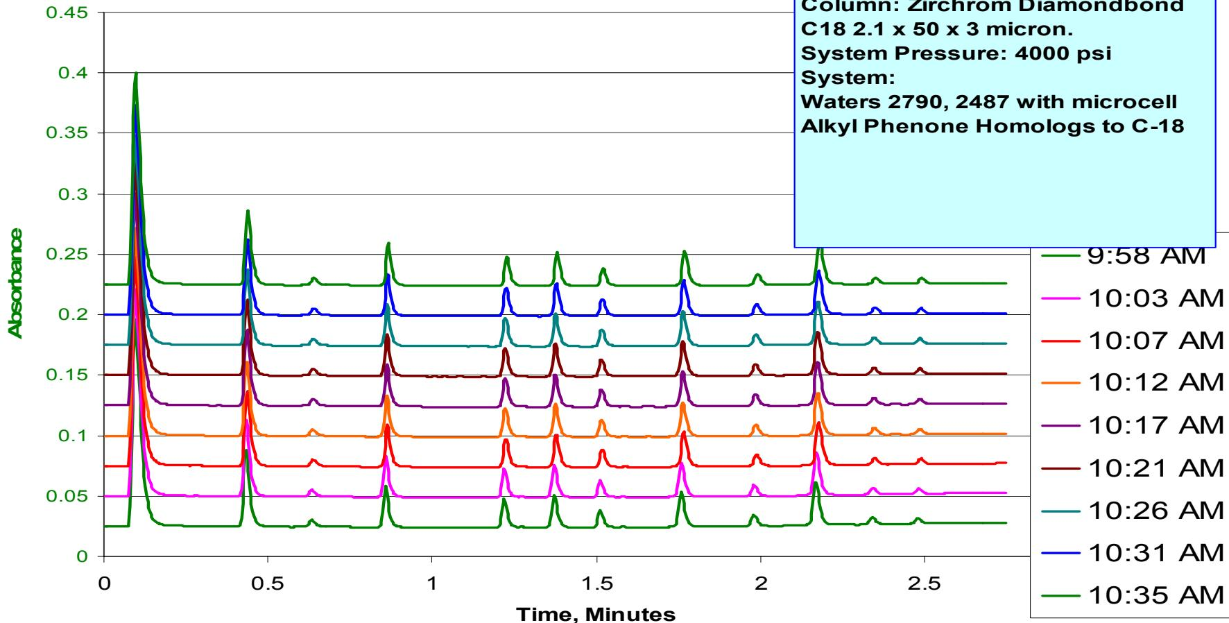
17 Gradients/Hour. Peak capacity is 70! This speed cannot be done at ambient within the gradient space! Carl Sims—Systec.
