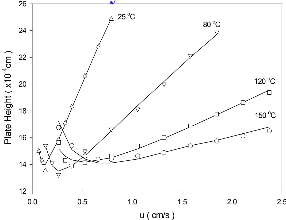
**Conclusion:** Resistance to mass transfer is **greatly reduced** at elevated column temperature.  $\Delta$ , 25 °C (decanophenone,  $k' = 12.23$ ),  $\nabla$ , 80 °C (dodecanophenone,  $k' = 7.39$ ),  $\square$ , 120 °C (tetradecanophenone,  $k' = 12.32$ ).
