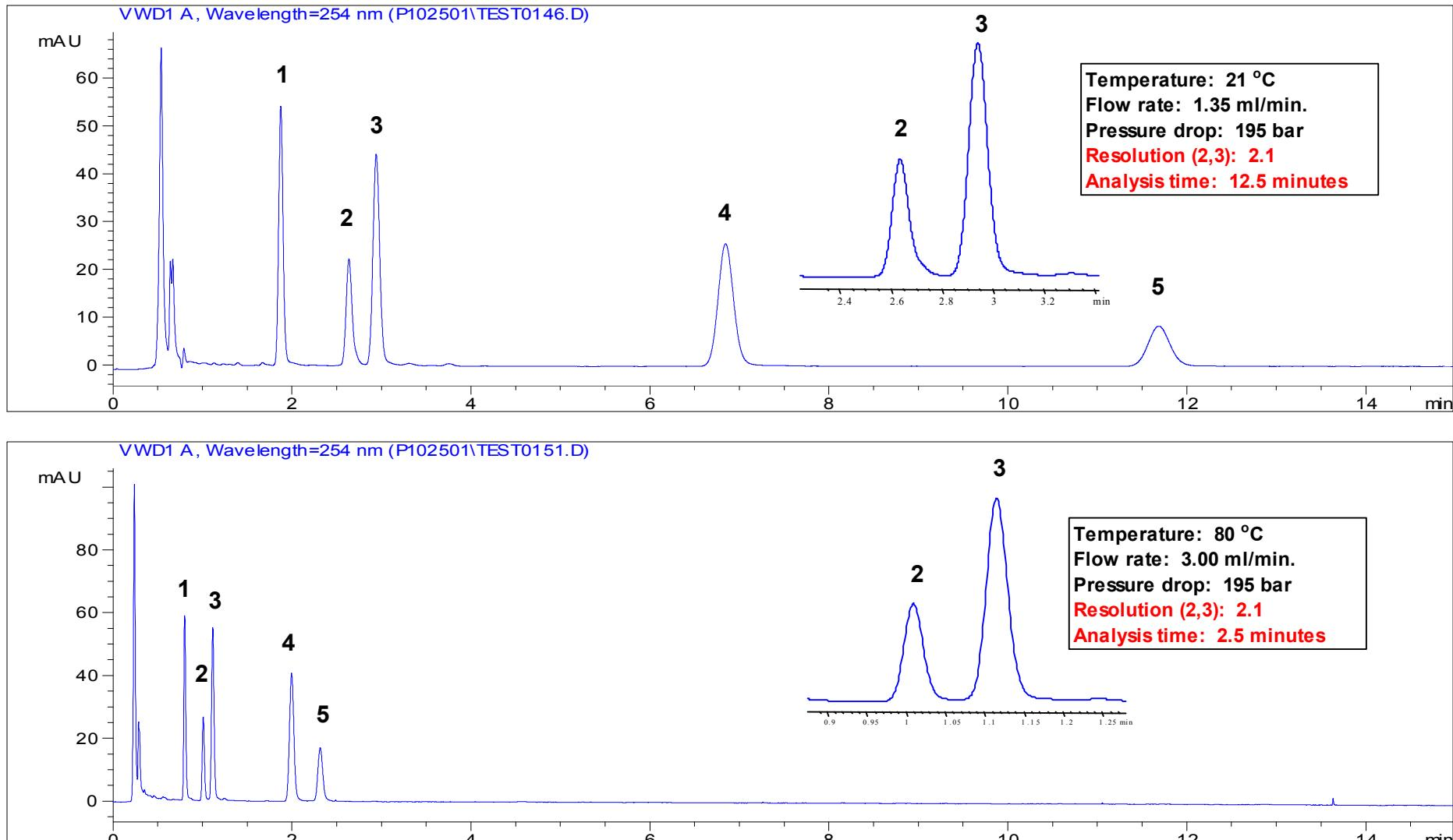
LC Conditions: (A) Mobile Phase, 29/71 ACN/50mM Tetramethylammonium hydroxide, pH 12.2; Flow Rate, **1.35 mL/min.**; Injection volume, 0.5  $\mu$ l; 254 nm detection; Temperature, **21°C**; Pressure drop = 195 bar; Solutes: 1=Doxylamine, 2=Methapyrilene, 3=Chlorpheniramine, 4=Triprolidine, 5=Meclizine
