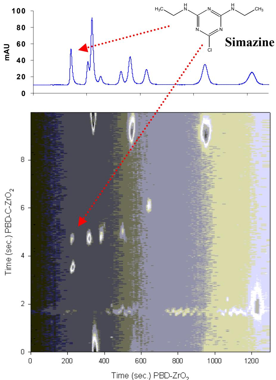
**1<sup>st</sup> Dimension Conditions:** Column, 50 mm x 2.1 mm i.d. PBD-ZrO<sub>2</sub>; Mobile phase, 20/80 ACN/Water; Flow rate, 0.08 ml/min.; Injection volume, 20 µl; Temperature, 40 °C
