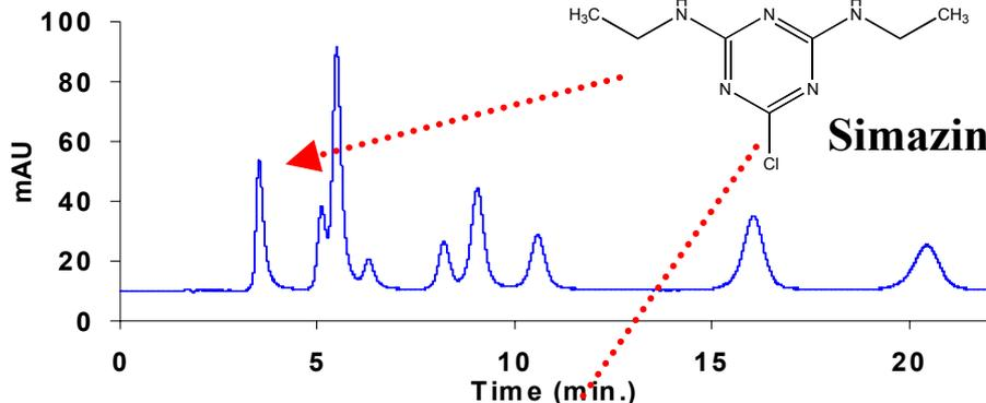
**1<sup>st</sup> Dimension Conditions:** Column, 50 mm x 2.1 mm i.d. PBD-ZrO<sub>2</sub>; Mobile phase, 20/80 ACN/Water; Flow rate, 0.08 ml/min.; Injection volume, 20 μl; Temperature, 40 °C
