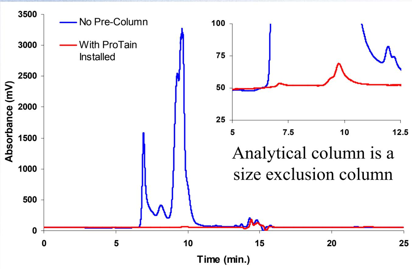
**LC Conditions:** Mobile phase, 20mM phosphate buffer, pH 6.8; Flow rate, 1.0 ml/min.; Temperature, ambient; Injection volume, 10  $\mu$ l.
