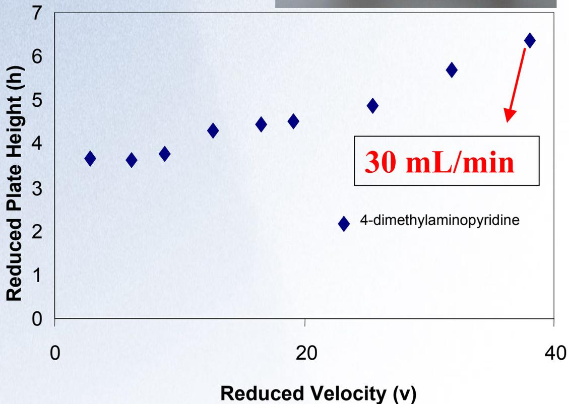
Rigid zirconia particles can withstand high pressure and high linear flow velocities.
