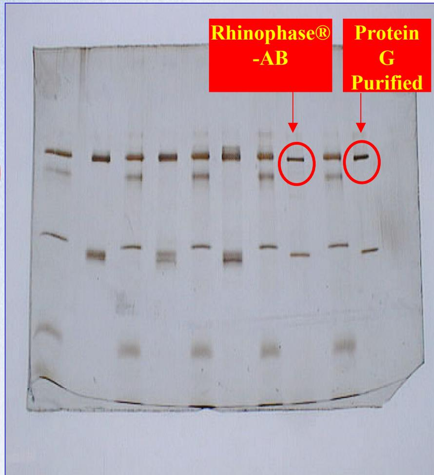
Silver-stained, SDS-PAGE gel Comparing IgG<sub>1</sub> purified by Protein G (row 1 from right) and Rhinophase®-AB (row 3 from right). Electrophoresis was run under reducing conditions. Sample loading at 1  $\mu$ g per lane. All other lanes are standards.
