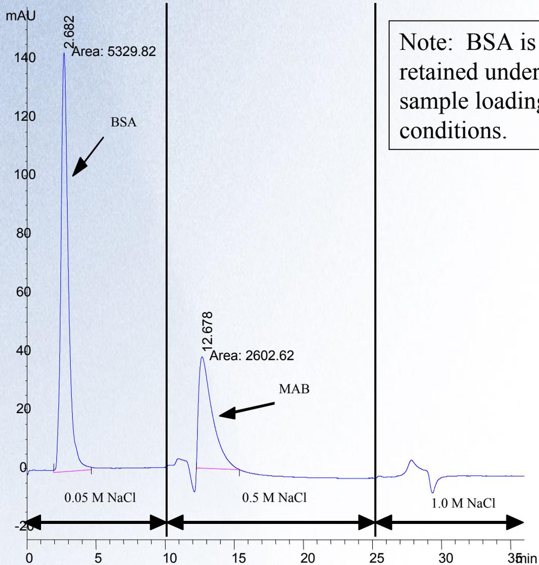
LC Conditions: 100  $\mu$ l injection of BSA (6.0 mg/ml) contaminated MAB (1.0 mg/ml) eluted by salt step gradient. Mobile phase: 20 mM MES, 4 mM EDTPA, 0.05 M-to-1.0 M NaCl pH=5.5. Flow rate: 2.0 ml/min. Temperature: 30°C. Detection: 280 nm.
