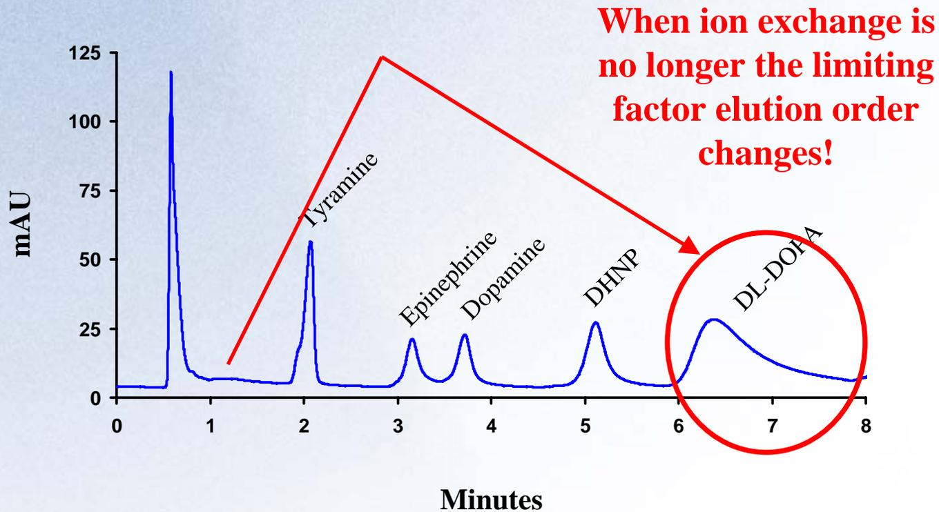
Conditions: ZirChrom® -PBD 50 mm x 4.6 mm, 85/15 ACN/10 mM Ammonium dihydrogen phosphate, 30 mM Ammonium Acetate pH=3.4, Flow=1.5 ml/min , Temperature =35° C, Detection UV= 254nm, 5 ul injection. Solute : Tyramine, Epinephrine, Dopamine, DHNP, DL-DOPA.
