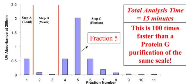
Step A = 20 mM MES buffer, 4 mM EDTPA, 50 mM NaCl @ pH 4.0, Step B = 20 mM MES buffer, 4 mM EDTPA, 50 mM NaCl @ pH 4.0, Step C = 20 mM MES buffer, 4 mM EDTPA, 2.0 M NaCl @ pH 4.0. Flow Rate = 60 mL/min, Injection size = 31.6 mL serum-free cell culture supernatant diluted 4-times with loading buffer, (3.98 mg of Mab), Amount of Rhinophase<sup>®</sup>-AB in tube = 10 grams.
