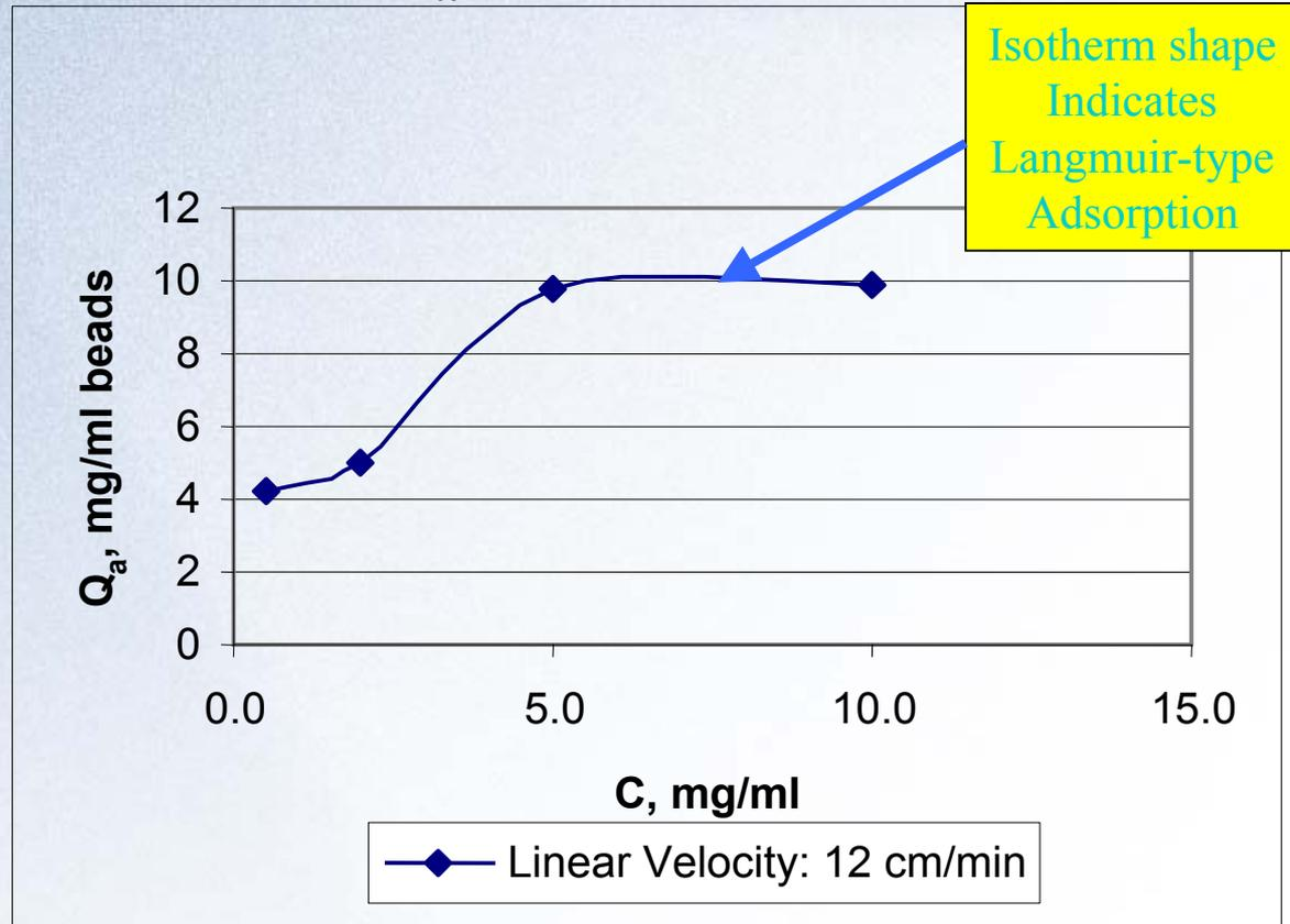
Conditions: Pure hIgG in Loading Buffer (20mM MES, 4mM EDTPA, 50mM NaCl, pH5.5) was loaded on a 5x4.6mm i.d. ZirChrom Mab Media column at a linear velocity of 12.0cm/min and detected at 280nm. The injection was continued until the absorbance of the effluent reached 80% of the inlet concentration. The column was then washed with Loading Buffer until it had reached baseline. The Adsorbed hIgG was then eluted with Elution Buffer (20mM MES, 4mM EDTPA, 1.0M NaCl, pH5.5).
