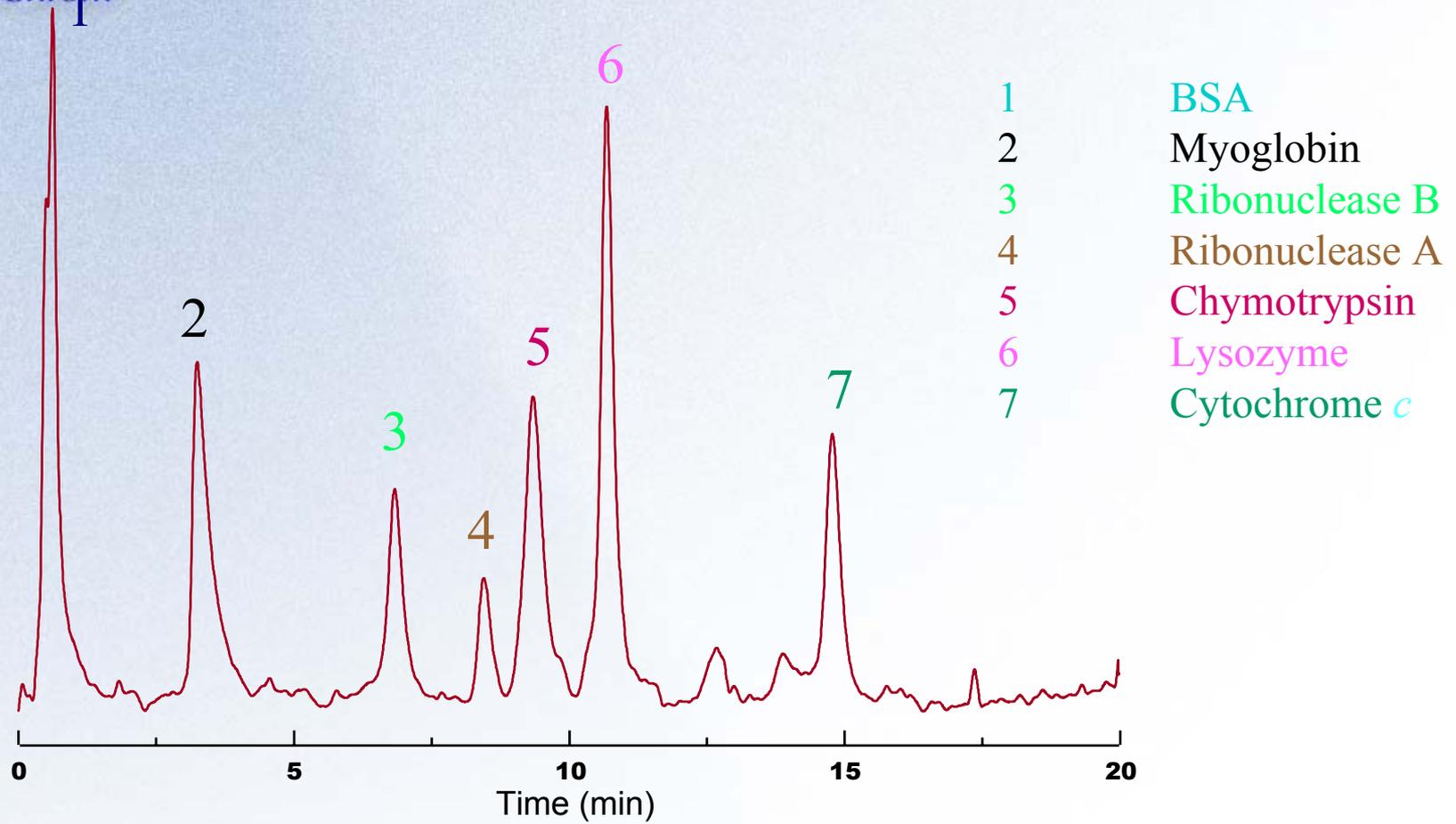
Protein mixture. Mobile phase: 4 mM P-EDTA, 20 mM MES, pH 5.5; linear gradient from 0 to 1 M Na<sub>2</sub>SO<sub>4</sub> in 30 min. Flow Rate 1 mL/min. UV detection at 280 nm.
