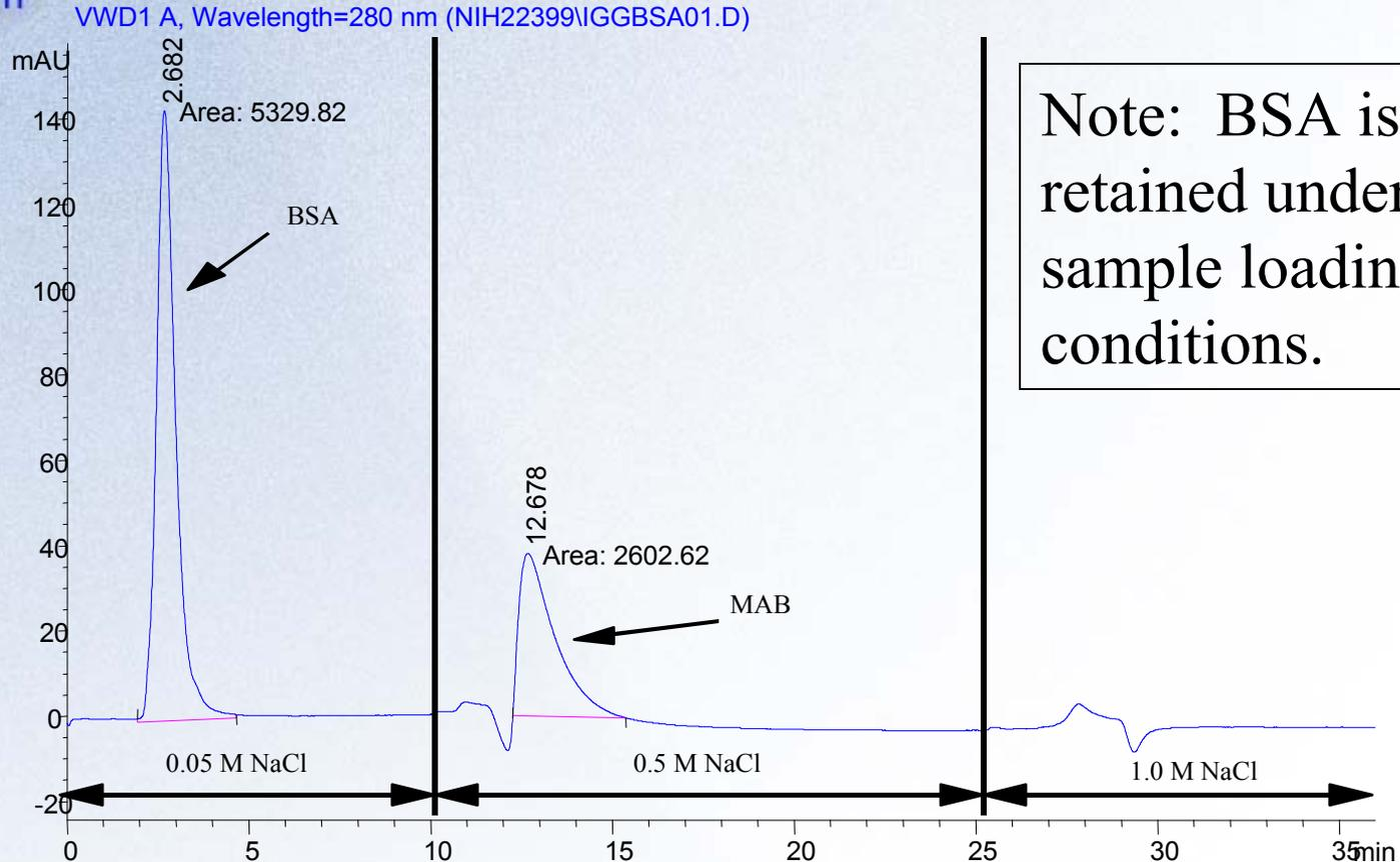
Note: BSA is not retained under sample loading conditions.
