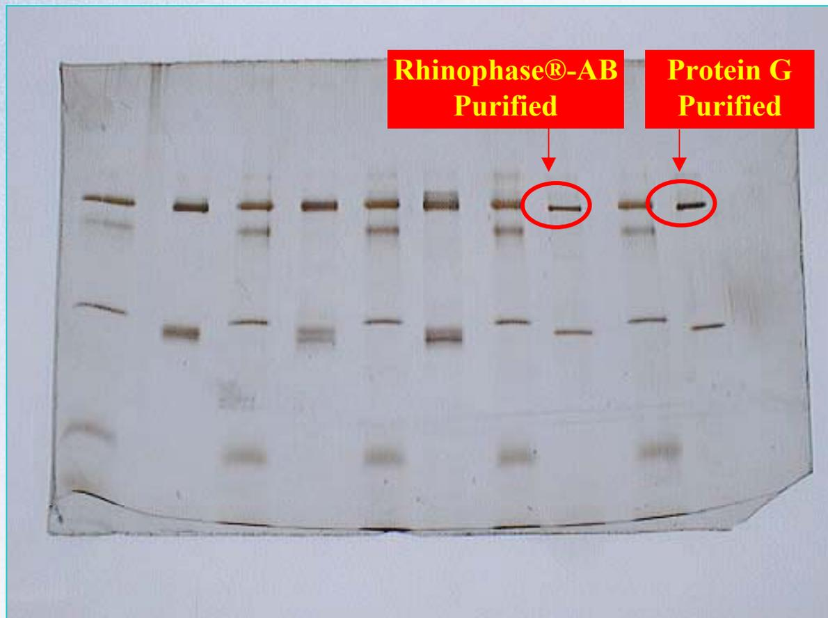
Silver-stained, SDS-PAGE gel Comparing IgG<sub>1</sub> purified by Protein G (row 1 from right) and Rhinophase®-AB (row 3 from right). Electrophoresis was run under reducing conditions. Sample loading at 1  $\mu$ g per lane. All other lanes are standards.
