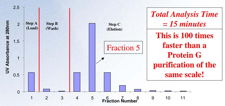
Step A = 20 mM MES buffer, 4 mM EDTPA, 50 mM NaCl @ pH 4.0, Step B = 20 mM MES buffer, 4 mM EDTPA, 50 mM NaCl @ pH 4.0, Step C = 20 mM MES buffer, 4 mM EDTPA, 2.0 M NaCl @ pH 4.0. Flow Rate = 60 mL/min, Injection size = 31.6 mL serum-free cell culture supernatant diluted 4-times with loading buffer, (3.98 mg of Mab), Amount of Rhinophase®-AB in tube = 10 grams.
