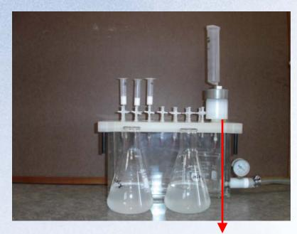
Vacuum manifold for loading the VersaFlash Column
