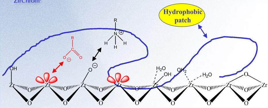
Three interactions acting simultaneously lead to irreversible adsorption of proteins on polymer coated zirconia materials
