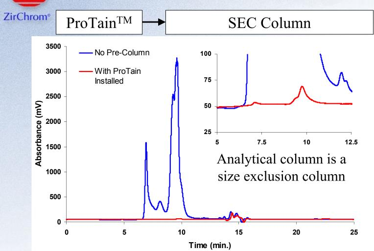
**LC Conditions**: Mobile phase, 20mM phosphate buffer, pH 6.8; Flow rate, 1.0 ml/min.; Temperature, ambient; Injection volume, 10 µl.
