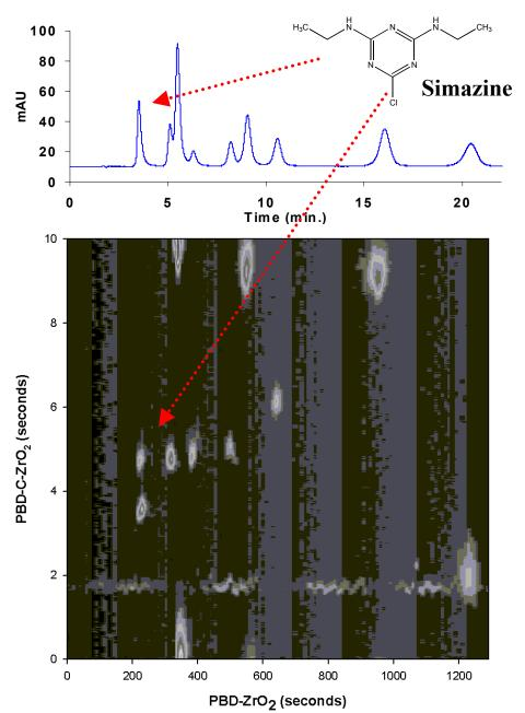
**1<sup>st</sup> Dimension Conditions**: Column, 50 mm x 2.1 mm i.d. PBD-ZrO<sub>2</sub>; Mobile phase, 20/80 ACN/Water; Flow rate, 0.08 ml/min.; Injection volume, 20 μl; Temperature, 40 °C
