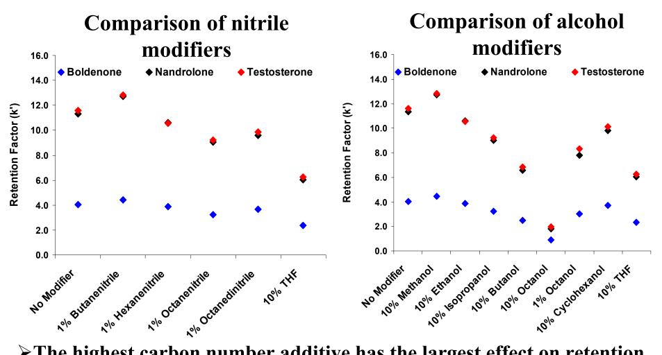
> The highest carbon number additive has the largest effect on retention
