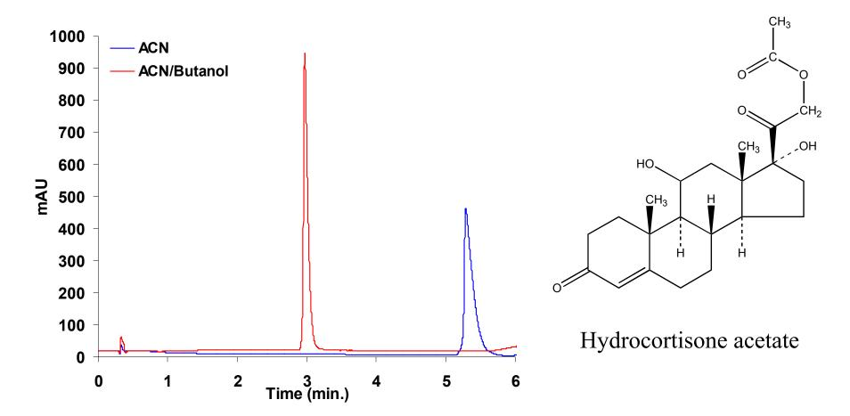
LC Conditions: Mobile phase, gradient elution from 10-90% of organic modifier from 0-5 minutes, with 20mM ammonium carbonate, pH 9.0 buffer; Flow rate, 2.0 ml/min.; Temperature, 80 °C; Injection volume, 1 µl; Detection at 240 nm; Column, 50 mm x 4.6 mm i.d. ZirChrom<sup>®</sup>-CARB
