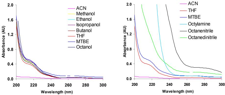
The relative similarity of the spectra for all mixtures containing HPLC grade solvents indicates that the very strongest solvent additive should be used, so that the relative amount of the additive can be reduced.
