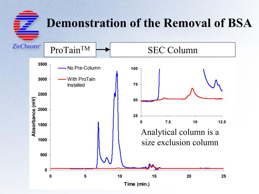
**LC Conditions**: Mobile phase, 20mM phosphate buffer, pH 6.8; Flow rate, 1.0 ml/min.; Temperature, ambient; Injection volume, 10 µl.
