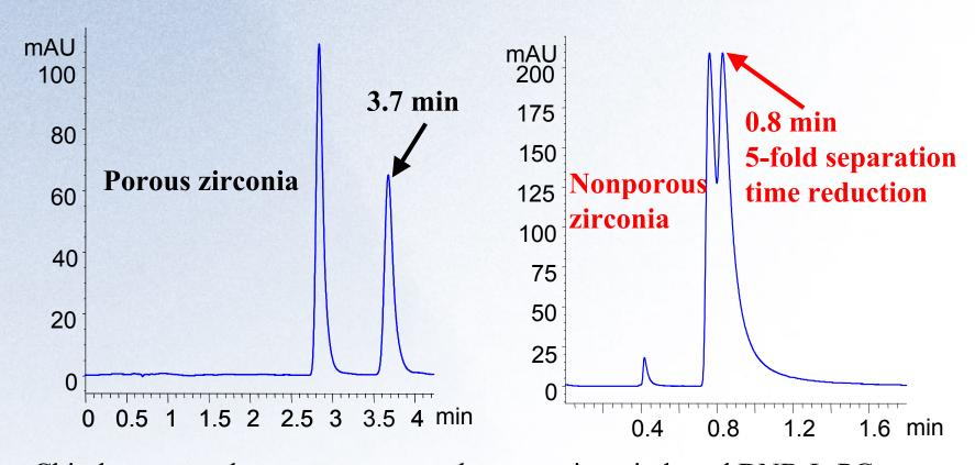
Chiral compounds on nonporous and porous zirconia-based DNB-L-PG anchored with APPA. Chromatographic conditions: mobile phase 99/1Hexane/IPA, probe solute: (±)trifluoroanthryl ethanol.
