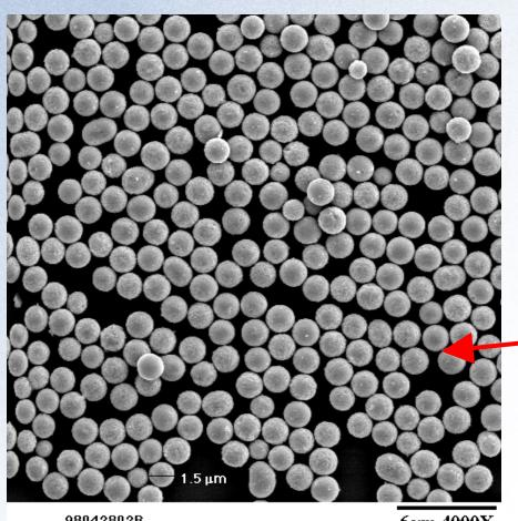
The resulting particles are monodisperse, spherical and nonaggregated.
