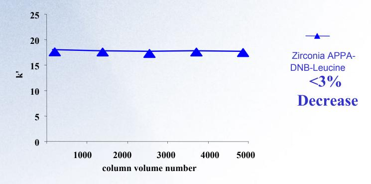
Flush Solvent: 49.5/49.5/1 Hexane/IPA/TFA Zirconia-based CSP is a very stable CSP.
