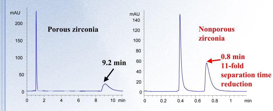
Chiral compounds on nonporous and porous zirconia-based DNB-L-Leu anchored with APPA. Chromatographic conditions: mobile phase 99/1Hexane/IPA, probe solute: (±)1-naphthyl leucine ester.
