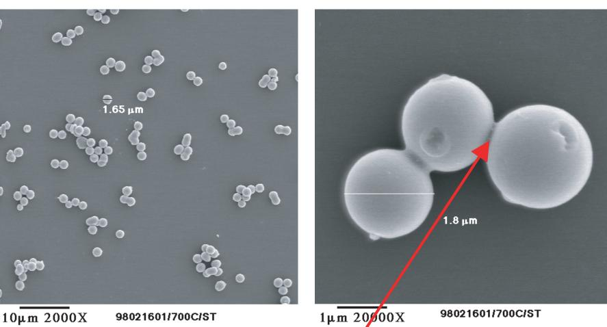
Collection by centrifugation causes "necks" and particle aggregation
