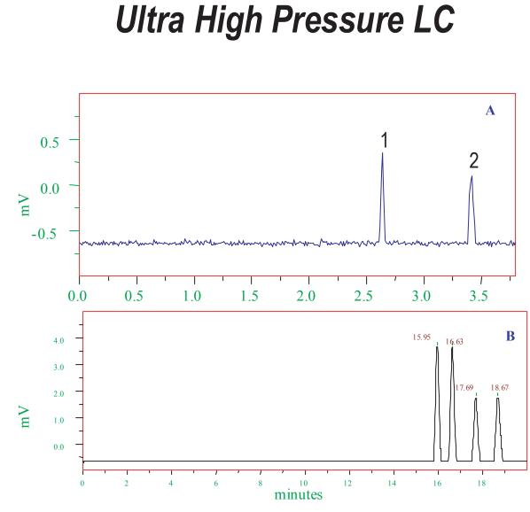
A: Separation of benzene (peak 1) and resorcinol (peak 2). Conditions: 5,000 psi inlet pressure; 25 cm x 75 micron i.d fused silica column packed with 2.0 micron PBDcoated nonporous zirconia; water/acetonitrile (64:40, v/v). Plate number for benzene is 61,000 N/m.
