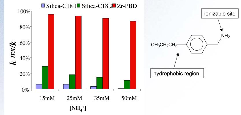
Conditions: 55% CH<sub>3</sub>OH in ammonium phosphate (pH, 6.0); 35°C; 1.0 mL/min.; UV 254 nm
