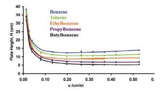
**Figure 2.** Plate height for Sub-2µm ZirChrom<sup>®</sup>-PBD based on van Deemter equation vs. linear velocity for alkylbenzenes; Mobile phase: 50/50 ACN/water (adjusted to keep k' constant in comparison to 3um particles)
