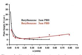
**Figure 3.** Plate height comparison for 3  $\mu$ m and Sub-2 $\mu$ m ZirChrom<sup>®</sup>-PBD based on van Deemter equation vs. linear velocity for alkylbenzenes; Mobile phase: 55/45 ACN/water
