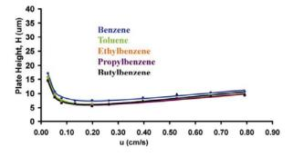
**Figure 1.** Plate height for 3µm ZirChrom<sup>®</sup>-PBD based on van Deemter equation vs. linear velocity for alkylbenzenes; Mobile Phase: 55/545 ACN/water
