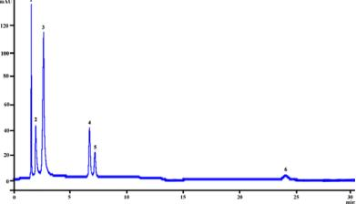
**Figure 2**: 1=Isopropylamine 2=Unknown 3=Glyphosate 4,5=peak D isomers 6=peak C (Impurity).
