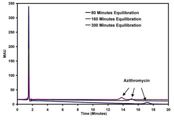
**Figure 3**: Affect of column exposure to USP mobile phase (equilibration) on the retention time of azithromycin.
