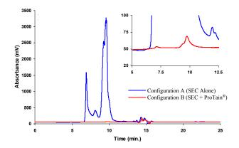
Figure 1. UV traces at 215 nm of the elution of BSA from a SEC column with and without ZirChrom's ProTain<sup>®</sup> system installed.
