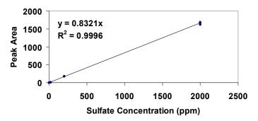
Figure 2: Standard Curve for Sulfate Analysis on ZirChrom<sup>®</sup>-SAX
