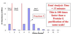
Step A = 20 mM MES buffer, 4 mM EDTPA, 50 mM NaCl @ pH 4.0, Step B = 20 mM MES buffer, 4 mM EDTPA, 50 mM NaCl @ pH 4.0, Step C = 20 mM MES buffer, 4 mM EDTPA, 20 m NaCl @ pH 4.0. Step C = 20 mM MES buffer, 4 mM EDTPA, 2.0 m NaCl @ pH 4.0. Flow Rate = 60 mL/min, Injection size = 31.6 mL serum-free cell culture supernatant diluted 4-times with loading buffer, (3.98 mg of Mab), Amount of Rhinophase\*-AB in tube = 10 grams.
